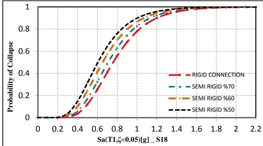
Fig.7.collaps Fragility curves of 18-story frame with IM=Sa ( $T_1$ ,  $\xi = 0.05$ )
