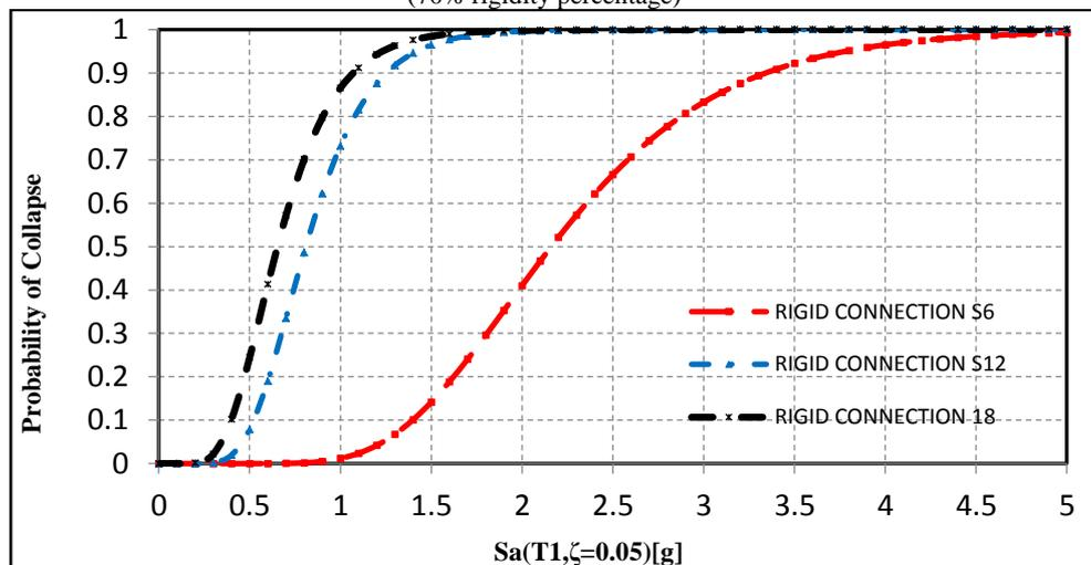
Fig. 10. Collapse fragility curves of 6-, 12- and 18-stories frame considering  $IM=Sa(T_1, \xi = 0.05)$  and semi-rigid connections (60% rigidity percentage)
