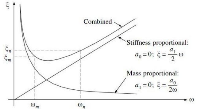
Fig.3. Relation between damping ratio and frequency for Rayleigh damping [17]
