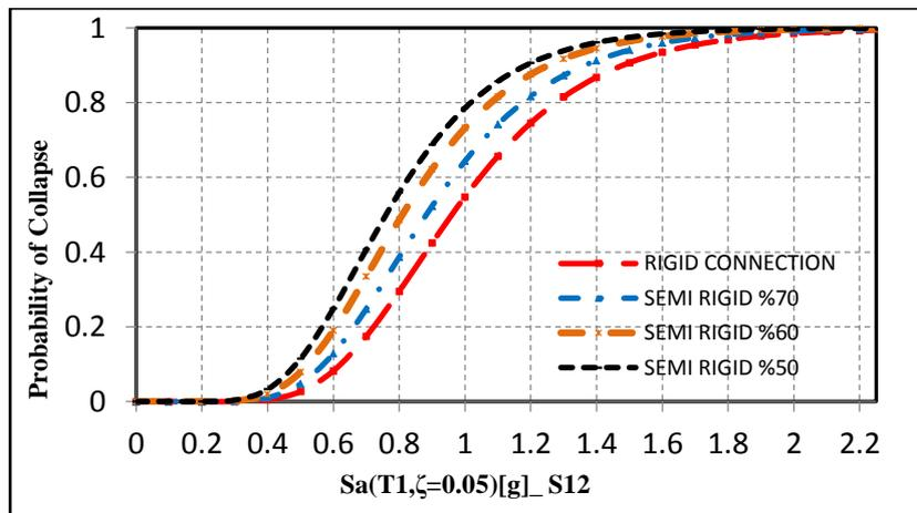
Fig.6. Collapse fragility curves of 12-story frame considering  $IM = Sa(T_1, \xi = 0.05)$
