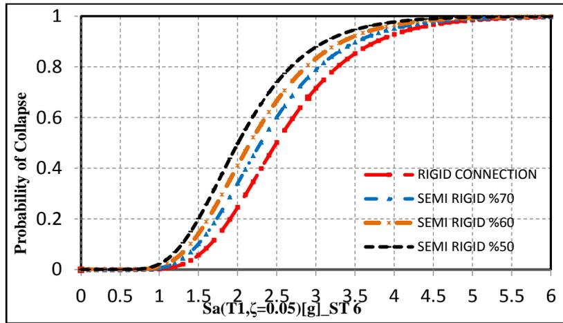
Fig.5. Collapse fragility curves of 6-story frame considering  $IM = Sa(T_1, \xi = 0.05)$
