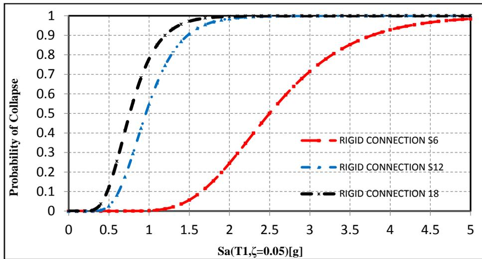
Fig. 8. Collapse fragility curves of 6-, 12- and 18-stories frame considering  $IM=Sa(T_1, \xi = 0.05)$  and rigid connections
