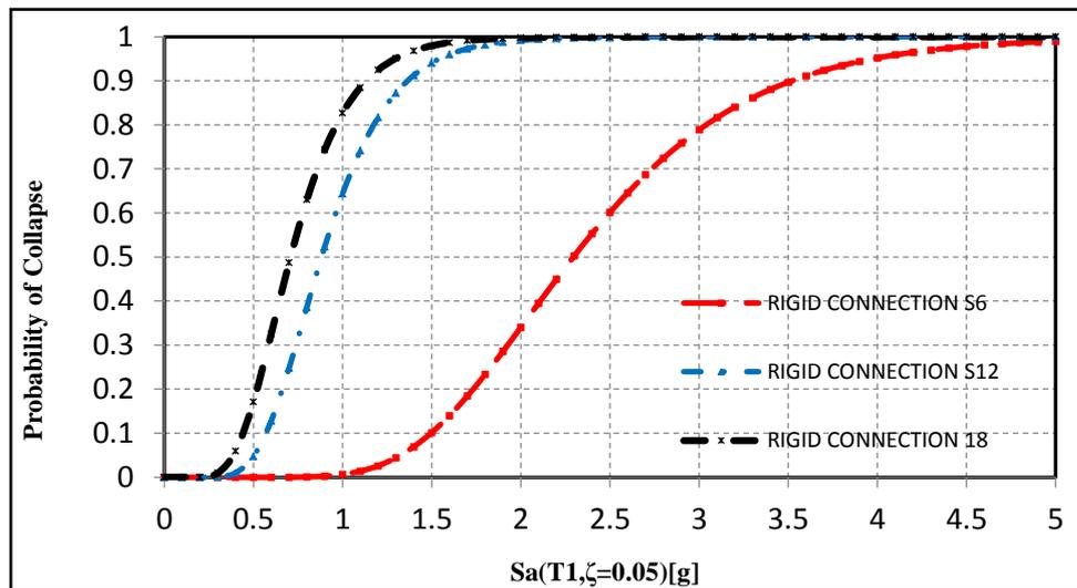
Fig. 9. Collapse fragility curves of 6-, 12- and 18-stories frame considering  $IM=Sa(T_1, \xi = 0.05)$  and semi-rigid connections (70% rigidity percentage)
