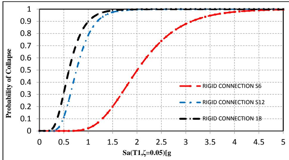
Fig.11. Collapse fragility curves of 6-, 12- and 18-stories frame considering  $IM=Sa(T_1, \xi = 0.05)$  and semi-rigid connections (50% rigidity percentage)
