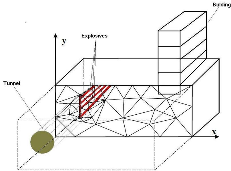
Fig. 1 Configuration of underground blast site
