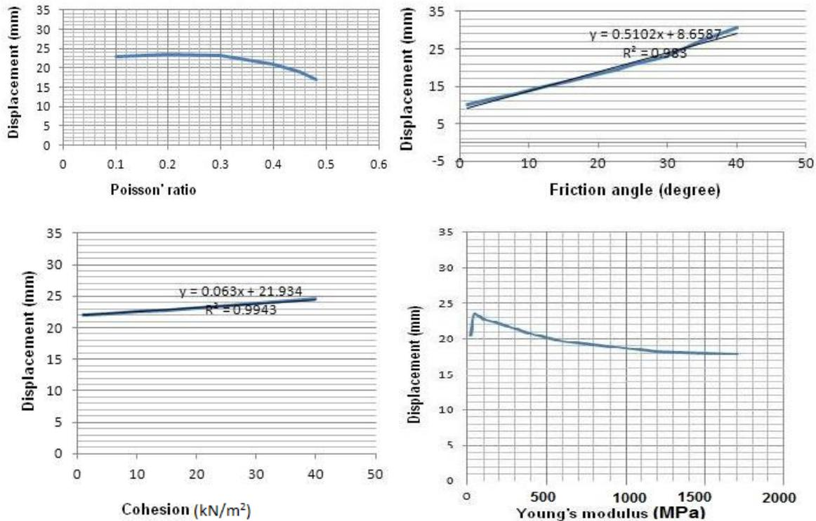
Fig. 5 The relationship between total displacement of the structure foundation and Poisson' ratio, Friction angle, Cohesion and Young's modulus of soil.
