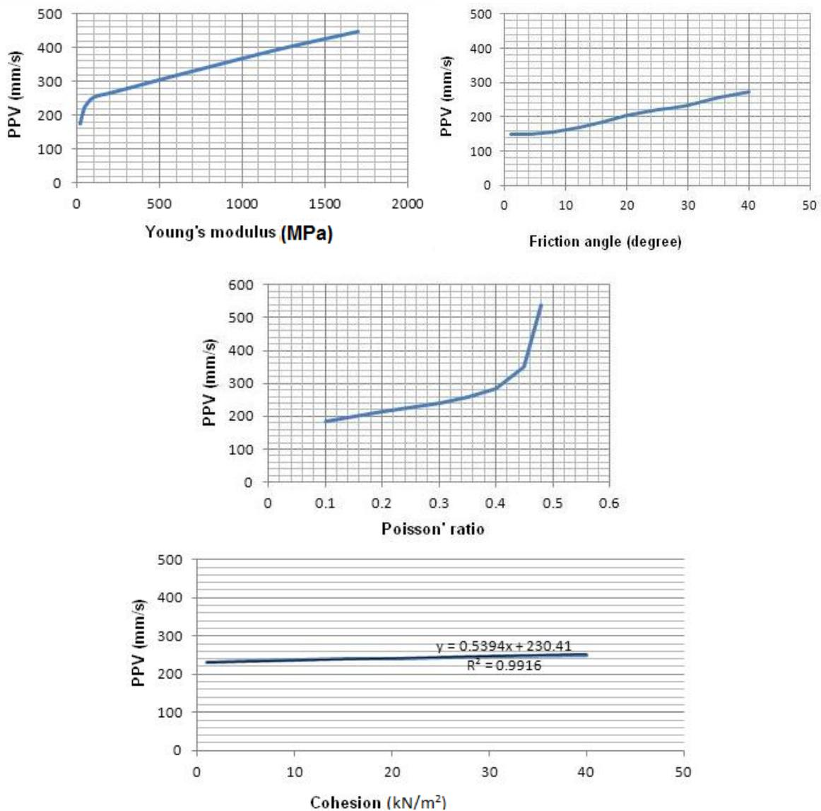
Fig. 4 The relationship between PPV in the structure foundation and Young's modulus, Friction angle, Poisson' ratio and Cohesion of soil.
