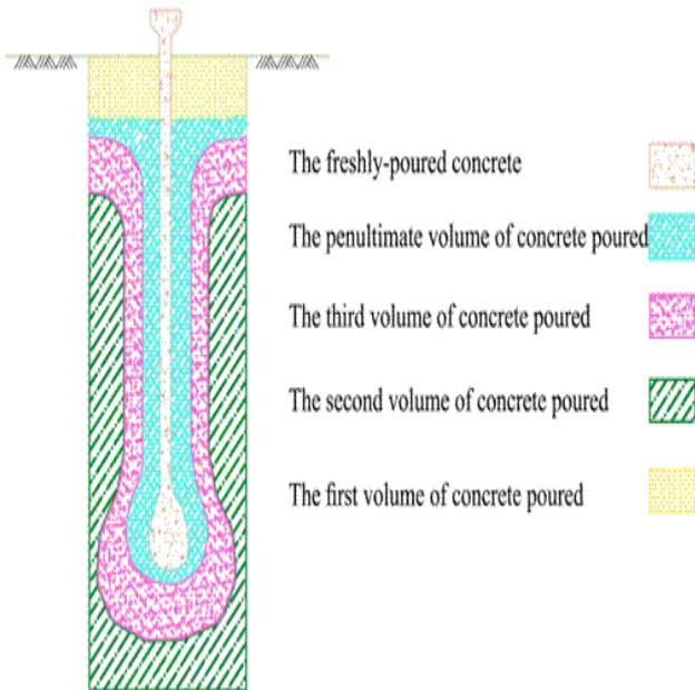
Figure 3- Concreting Section of the Modeled Panel using Color Concrete
