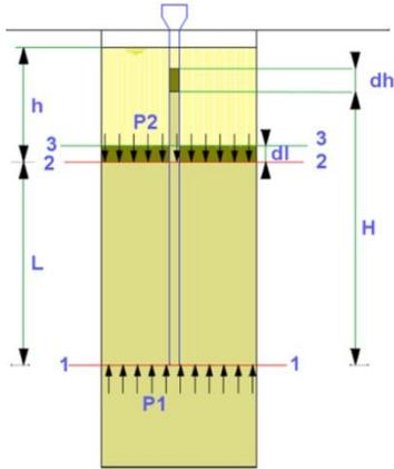
Figure 4- The Force of the Concrete and the Slurry Fluid in the Panel
