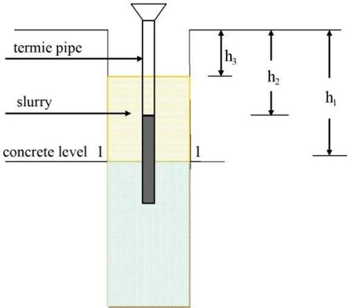
Figure 1- The static balance of the slurry and flow concrete
