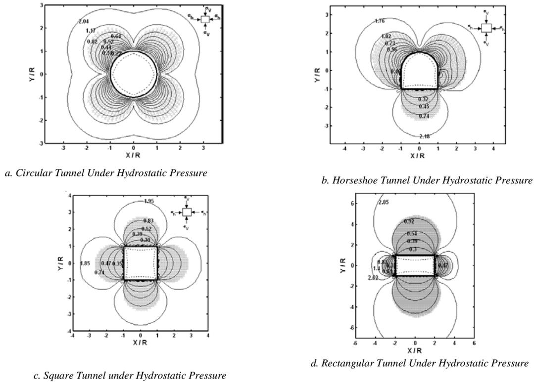
Figure 6. Failure zones around various sections of tunnel under hydrostatic compression
