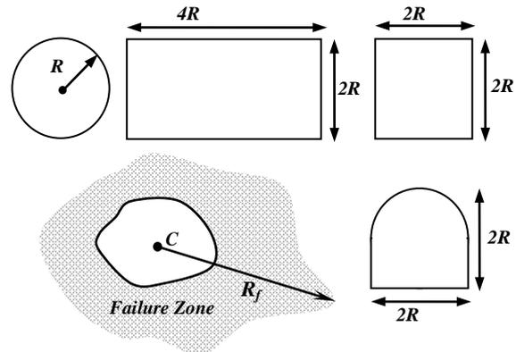
Figure 3. Assumed tunnel sections for determining failure zones
