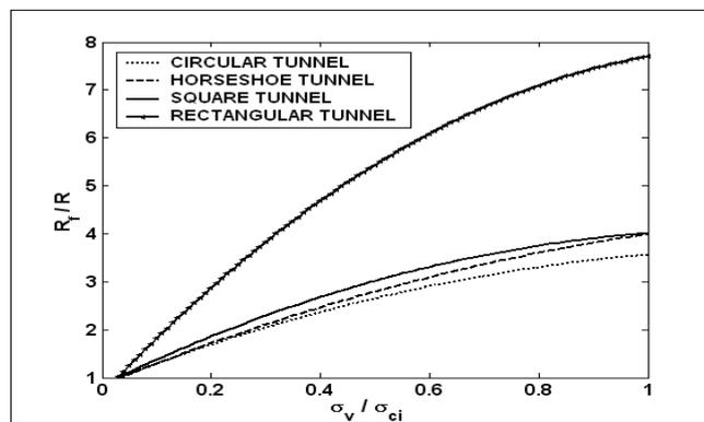
Figure 11. Comparison of tunnel section type in expansion of failure
