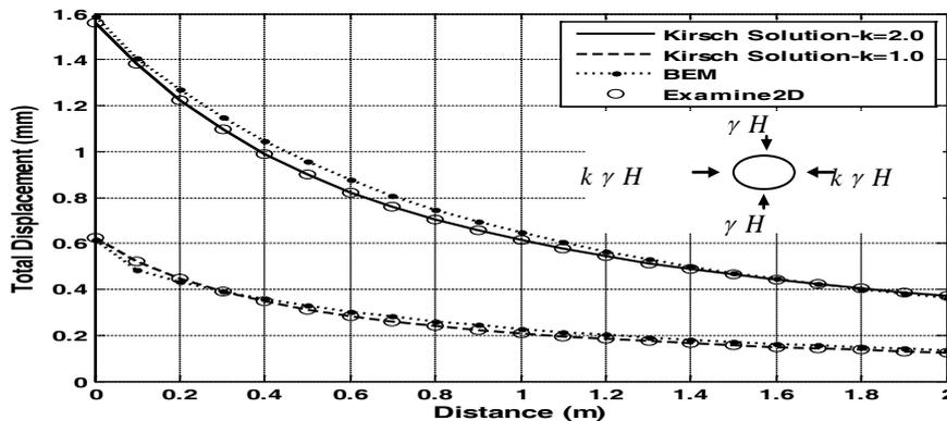
Figure 5. Comparison of total displacement values in different distances from the tunnel wall between analytical Solutions [12], EXAMINE<sup>2D</sup> software[13] and BEM(present study)
