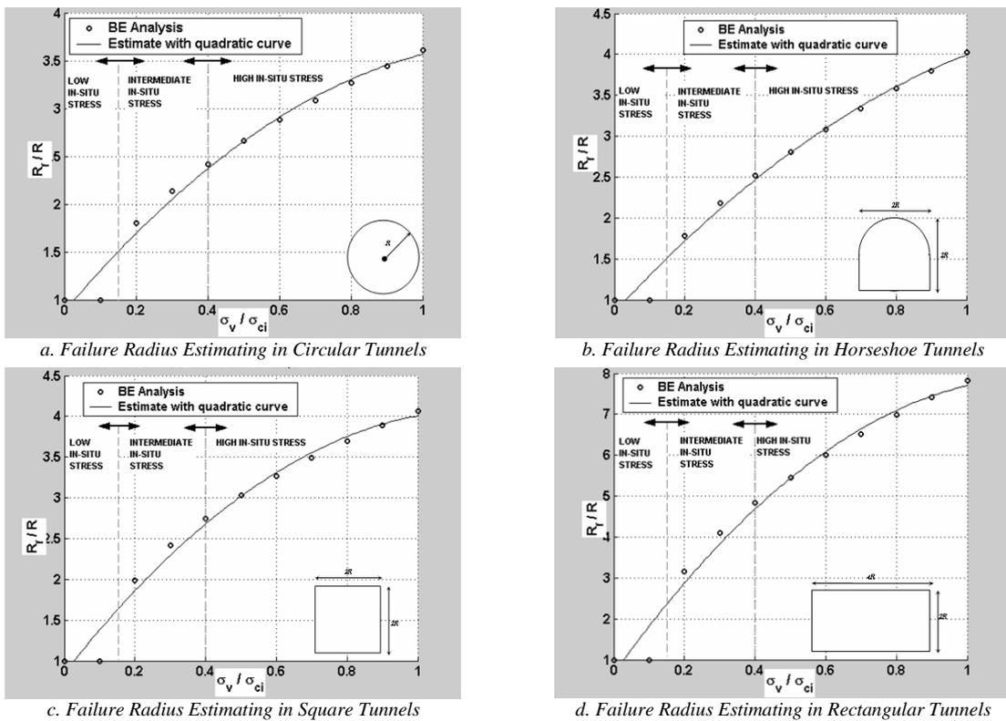
Figure 10. Failure behavior in various sections of tunnel for various values of insitu stresses
