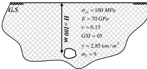
Figure 2. Properties of rock mass around tunnel
