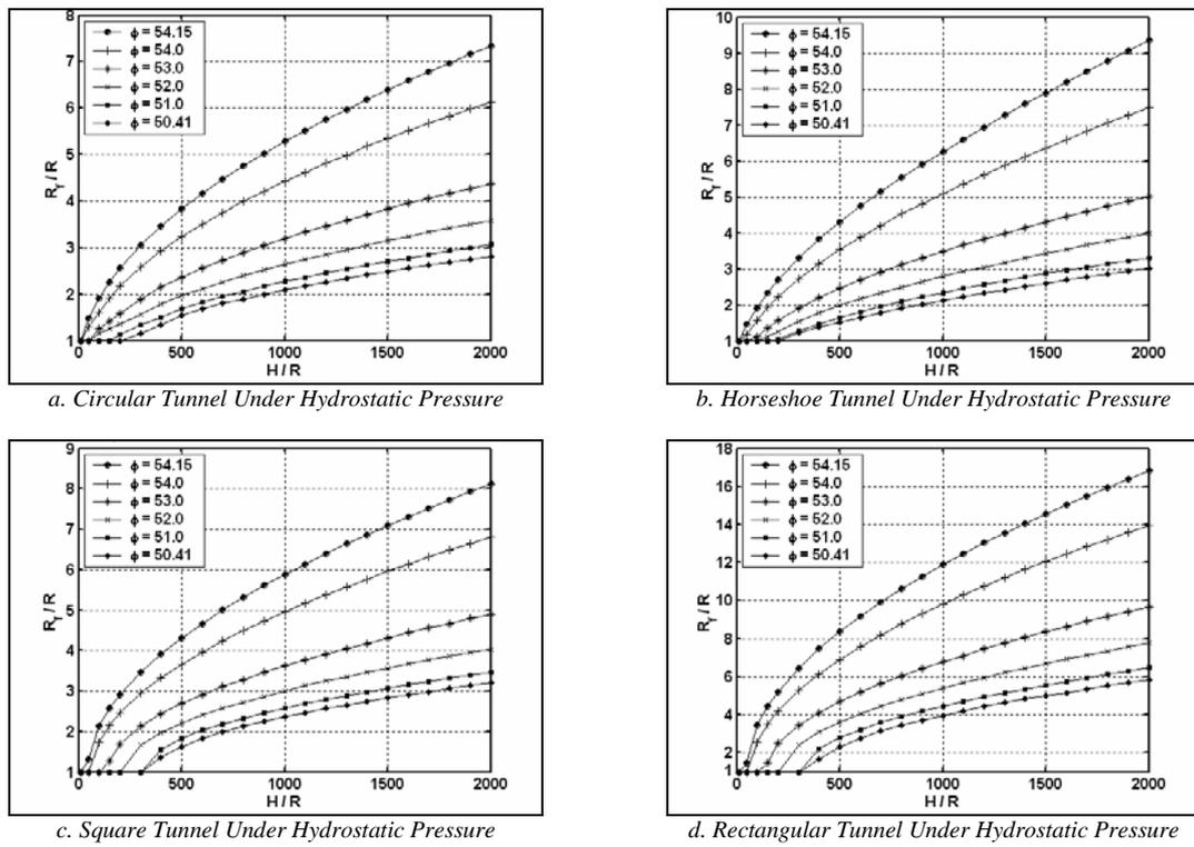
Figure 9. Expansion of failure radius in various condition of  $\Phi$
