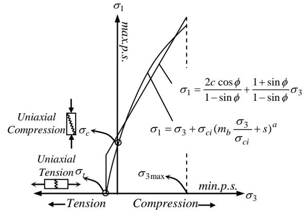
Figure 1. Relation between Hoek-Brown major and minor principle stresses and equivalency with Mohr-Colomb Criteria [4]
