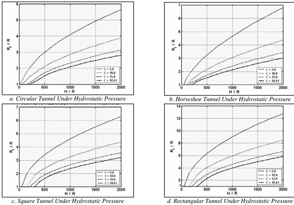
Figure 8. Expansion of failure radius in various cohesion values
