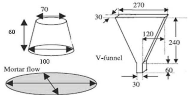
Fig. 2. Dimensions of mini-slump and mini V-funnel
