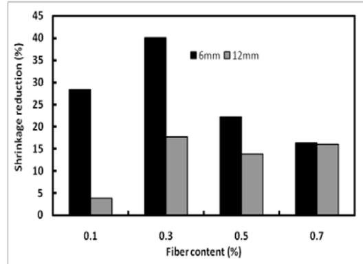
Fig. 10. Effect of PP fibers on shrinkage reduction after 180 days
