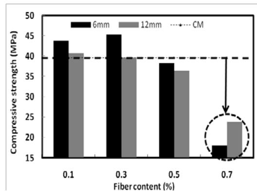
Fig. 11. Compressive strength of PP fiber reinforced SCM
