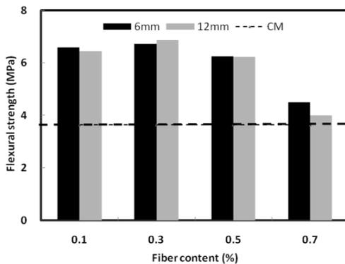
Fig. 13. Flexural strength of PP fibers reinforced SCM
