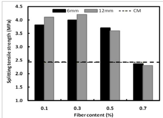
Fig. 12. Splitting tensile strength of PP fibers reinforced SCM
