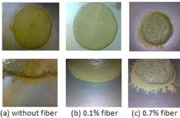
Fig. 7. Consistency of a mortar mixed with PP fiber with various fiber dosages
