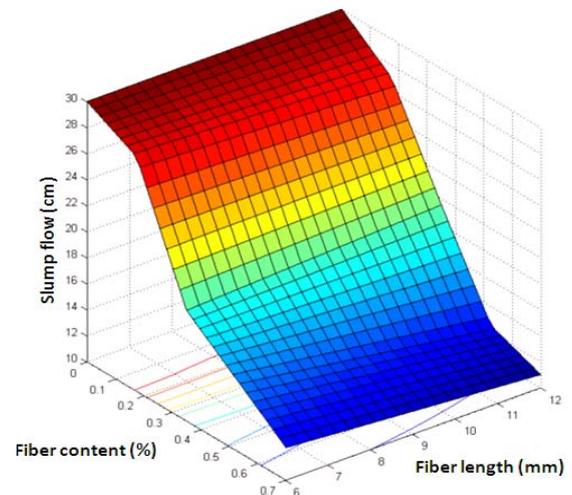
Fig. 4. Result of mini-slump test
