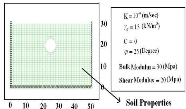
Fig. 3. Sketch of the model and soil properties
