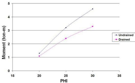
Fig. 4. Variations of bending moments versus friction angle (PHI) for drained and undrained conditions
