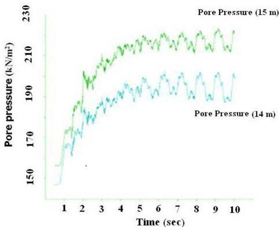
Fig. 11. Variations of pore pressure at the depths of 14 (m) and 15 (m) from ground surface (lower depths of tunnel crown,  $K=10^{-3}$  m/s)
