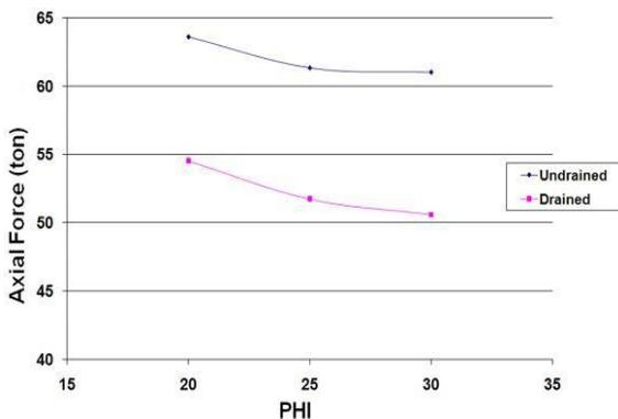
Fig. 5. Variations of axial forces versus friction angle (PHI) for drained and undrained conditions
