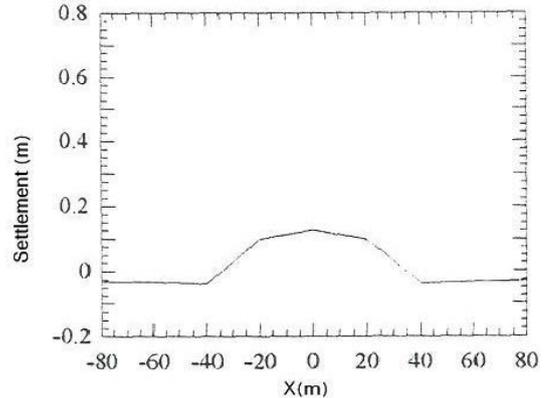
Fig. 2. Variation of surface deformation versus distance from the tunnel center
