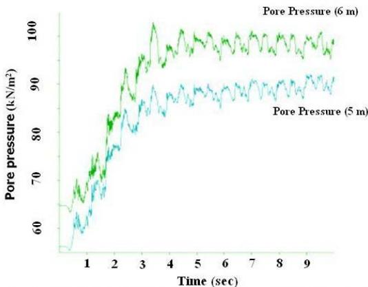
Fig. 8 Variations of pore pressure at the depths of 5 (m) and 6 (m) from ground surface (upper depths of tunnel crown,  $K= 10^{-4}$  m/s)
