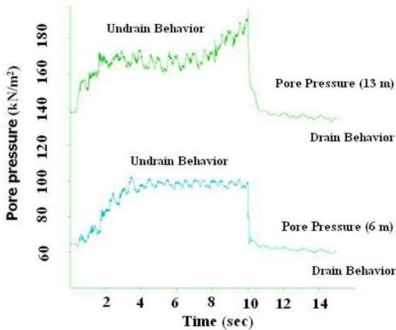
Fig. 7. Display of pore pressure variations in two points, upper depths of tunnel crown (at the depth of 6 m) and lower depths the tunnel (at the depths of 19 m) for drained and undrained conditions
