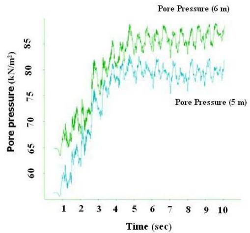
Fig. 9. Variations of pore pressure at the depths of 5 (m) and 6 (m) from ground surface (upper depths of tunnel crown,  $K= 10^{-3}$  m/s)
