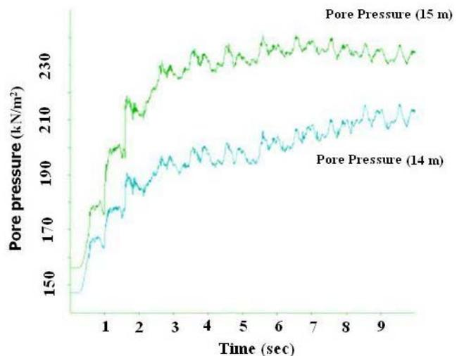
Fig. 10. Variations of pore pressure at the depths of 14 (m) and 15 (m) from ground surface (lower depths of tunnel crown,  $K= 10^{-4}$  m/s)
