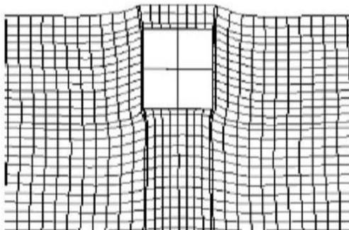
Fig. 1. Display of underground structure uplift due to the dynamic loading
