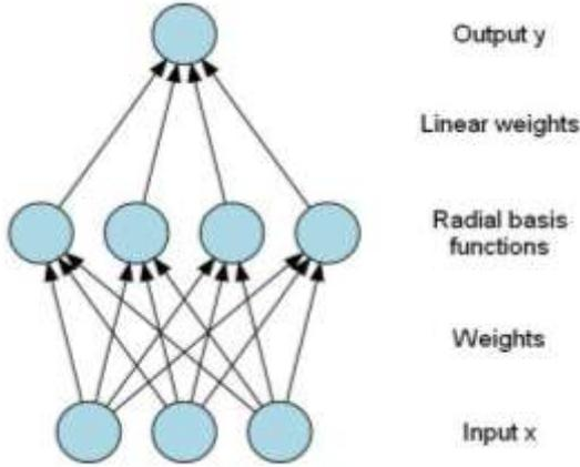
Fig.3. Structure of the radial basis function [27].
