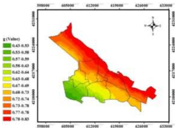
Fig 2. Seismic zonation map of Tabriz after amplification [6].
