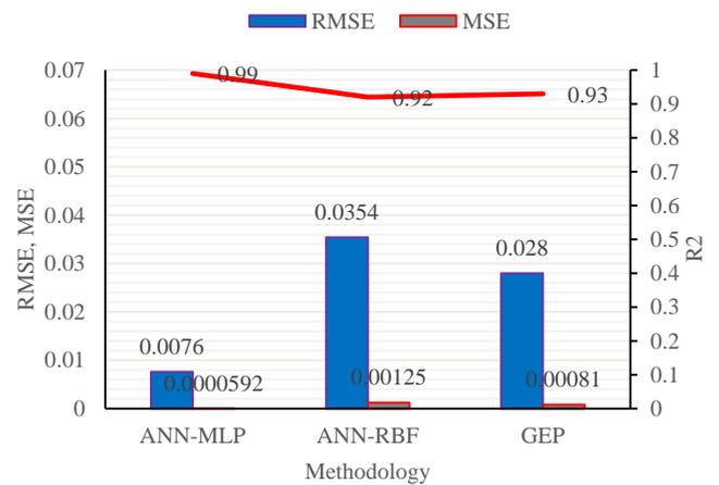
Fig.8. Comparison of  $R^2$ , RMSE and MSE statistical indices for accumulation energy ratios obtained from ANN-MLP, ANN-RBF and GEP modeling
