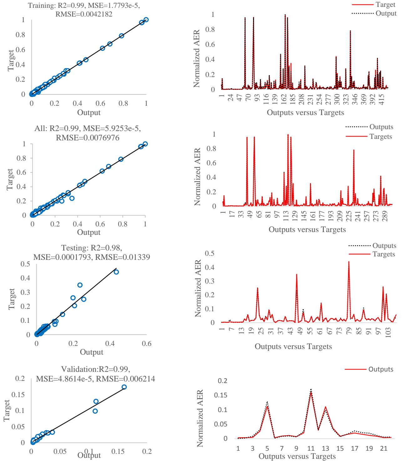
Fig.5. Results for estimating the accumulation energy ratio by the multilayer perceptron (MLP) function of the artificial neural network (ANN).
