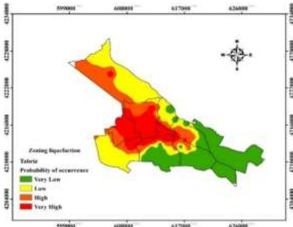
Fig.1. Zoning of the probability of liquefaction in Tabriz using the relation of accumulation energy ratio [6].
