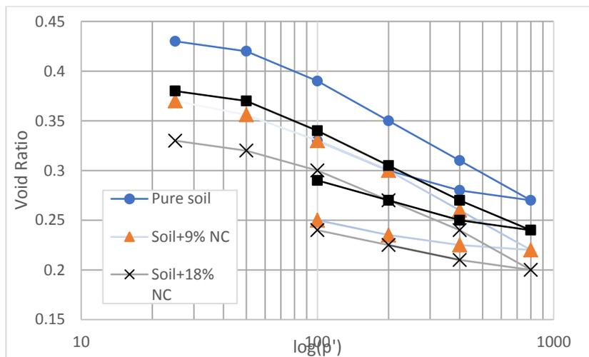
Fig.8. e-log curve of the consolidation test for Nano-CaCO<sub>3</sub> modified marl soils
