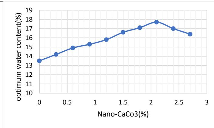
Fig.2. Variation of optimum water content marl soil modified with Nano-CaCo<sub>3</sub>
