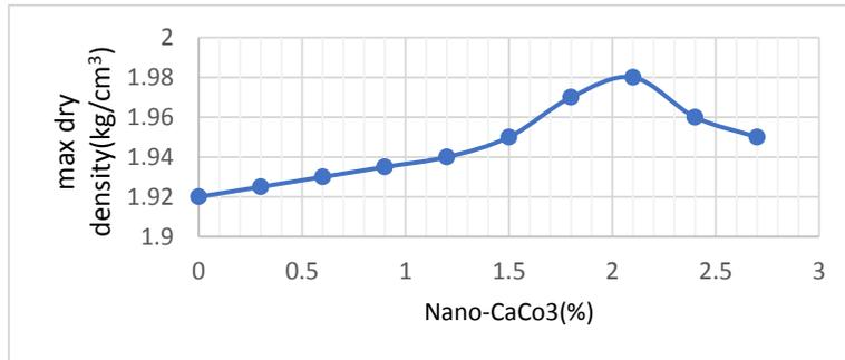
Fig.3. Variation of maximum dry density of marl soil modified with Nano-CaCo<sub>3</sub>
