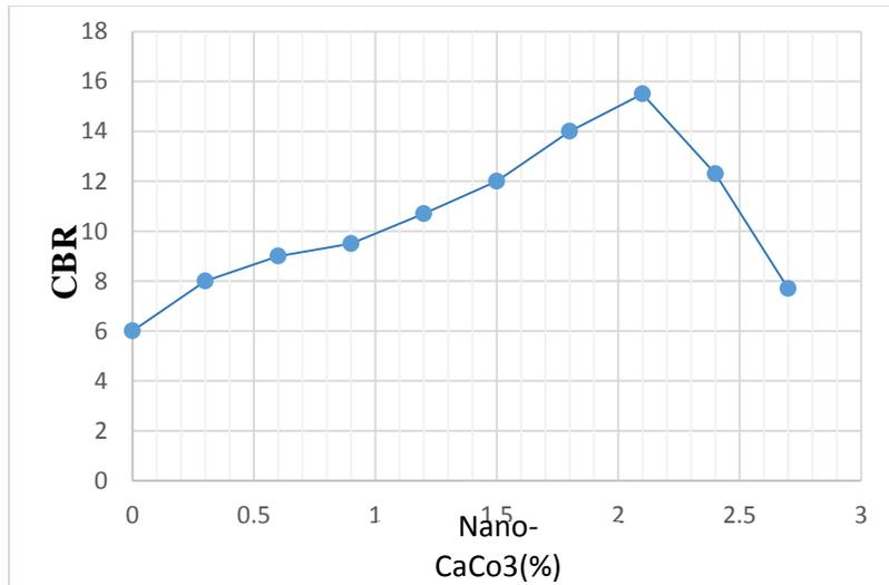
Fig.5.Variation of CBR of marl soil modified with Nano-CaCo<sub>3</sub>
