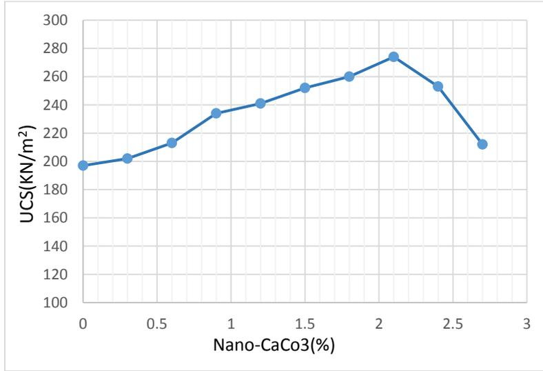
Fig.4. Variation of unconfined compression strength of marl soil modified with Nano-CaCo<sub>3</sub>
