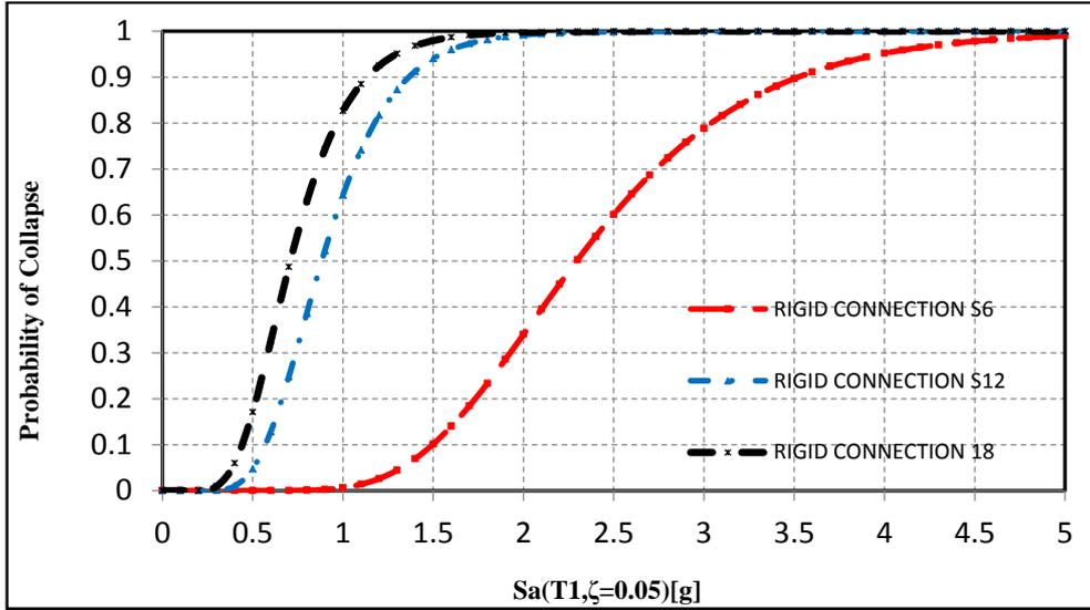
Fig 9. Collapse fragility curves of 6-, 12- and 18-stories frame considering  $IM=Sa(T_1, \zeta = 0.05)$  and semi-rigid connections (70% rigidity percentage)
