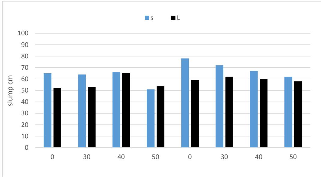
Figure 1. Slump comparison of specimens with LECA and scoria
