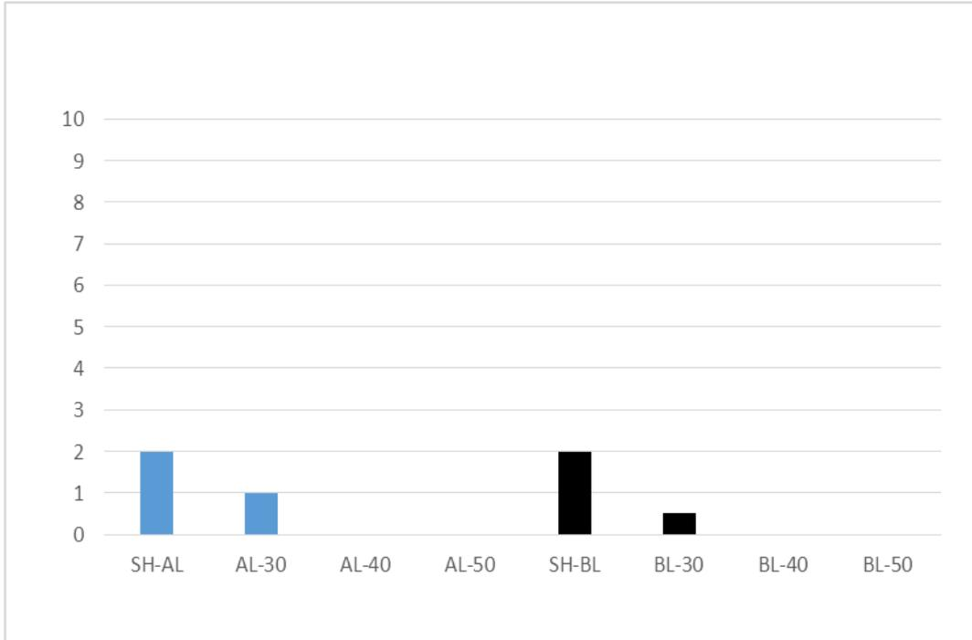
Figure 3. Difference between j-ring and slump results for mix designs with recycled LECA
