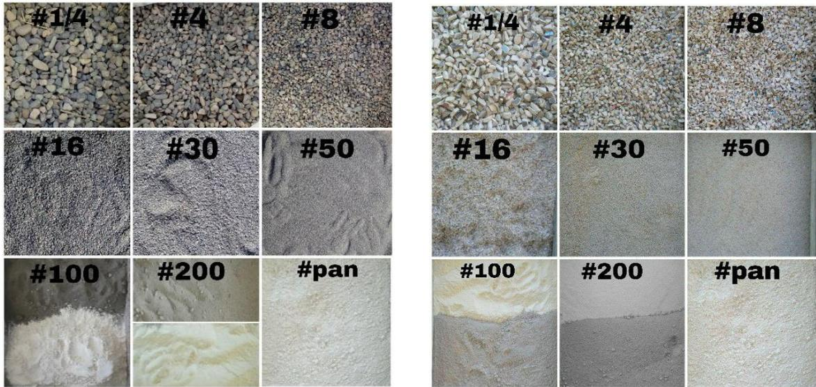
Figure 1. Grading of aggregates
