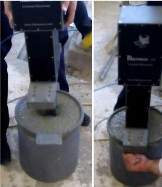
Figure 4. The rheometer test
