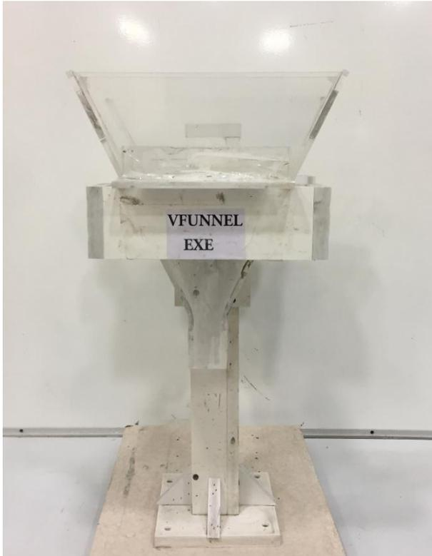
Figure 3. Configuration of mini V-funnel apparatus test.
