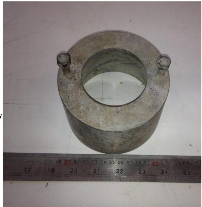
Figure 2. Configuration of mini-slump cone.
