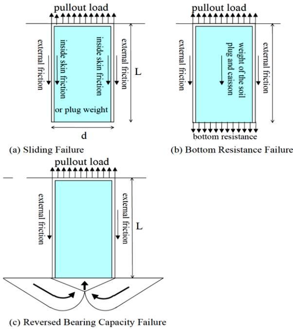
Figure 1. Failure modes for suction anchors under tensile loading [17]
