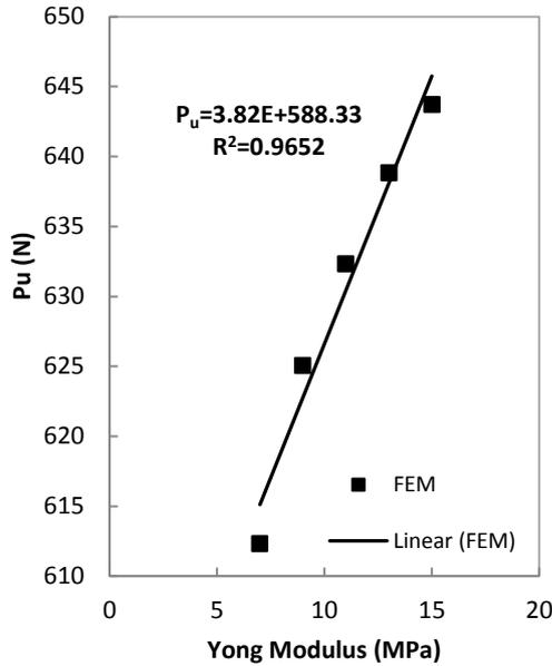
Figure 11. Yong modulus of soil on pull-out capacity of suction caissons
