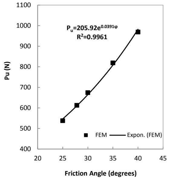
Figure 7. Soil friction angle on pull-out capacity of suction caissons
