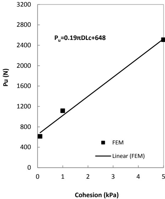
Figure 5. Soil cohesion effects on pull-out capacity of suction caissons
