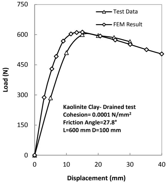
Figure 3. Comparison between the experimental [1] and FEM method
