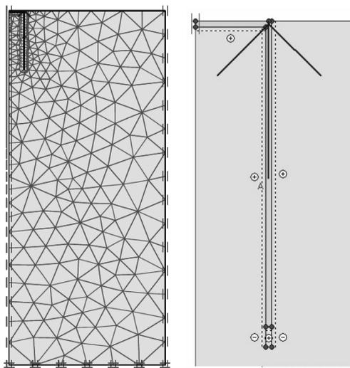
Figure 2. Finite element model and mesh generated
