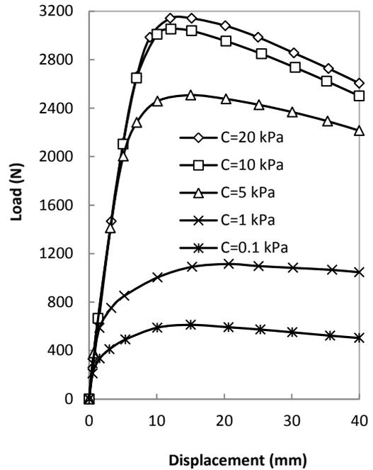
Figure 4. Soil cohesion effects on numerical pullout of suction caissons
