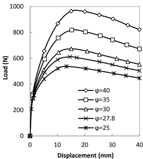
Figure 6. Soil friction angle on numerical pullout of suction caissons
