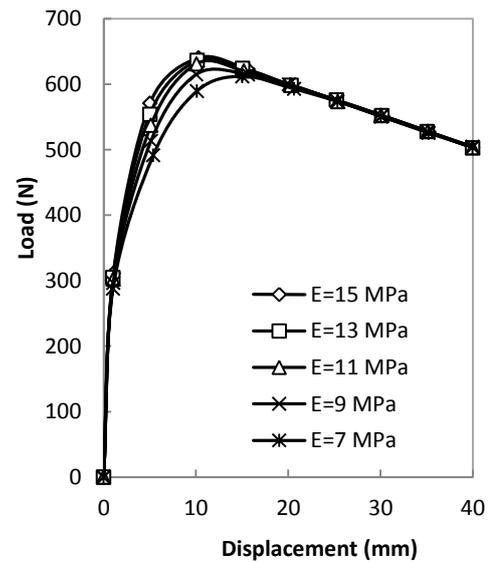
Figure 10. Yong modulus of soil on numerical pullout of suction caissons
