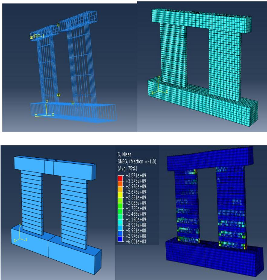
Figure 8. Shear wall modeling, stress, and meshing, in the sample C-2
