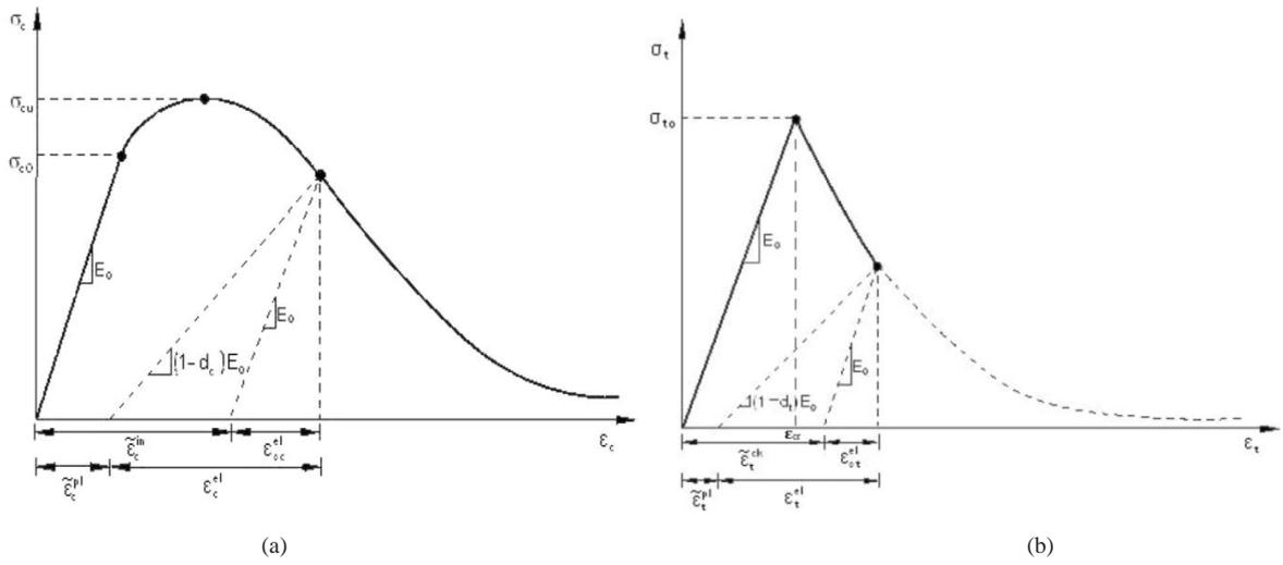
Figure 1. (a) Concrete compressive behavior (b) tensile behavior [26]
