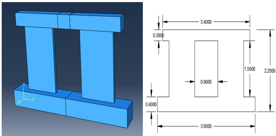
Figure 3. Dimensions of shear walls
