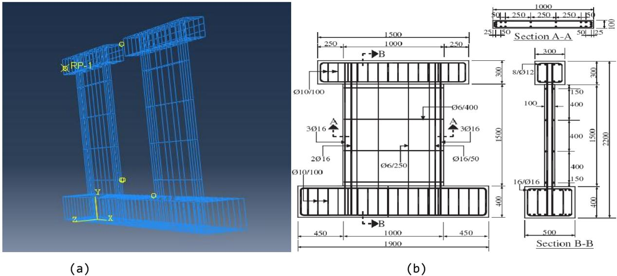
Figure 4. (a) Reinforcement details of test specimens (dimension in mm) [22] (b) Modeling of rebars in ABAQUS.
