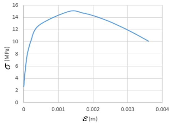
Figure 2. plastic stress-strain behavior of concrete
