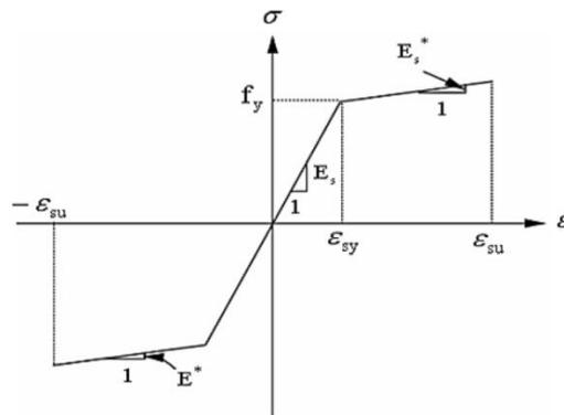
Figure 5. Bilinear behavior of steel.
