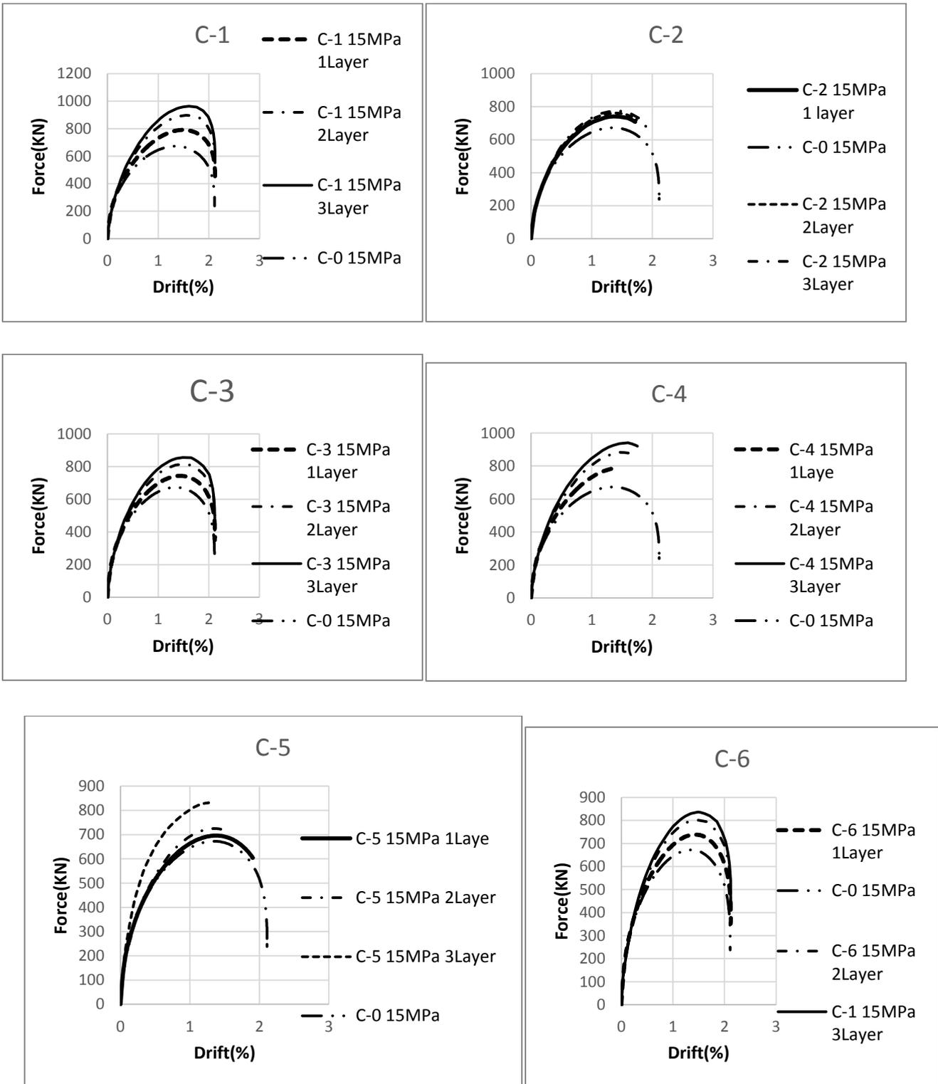
Figure 10. Load- Displacement curve for C-1, C-2, C-3, C-4, C-5, C-6 specimens configuration
