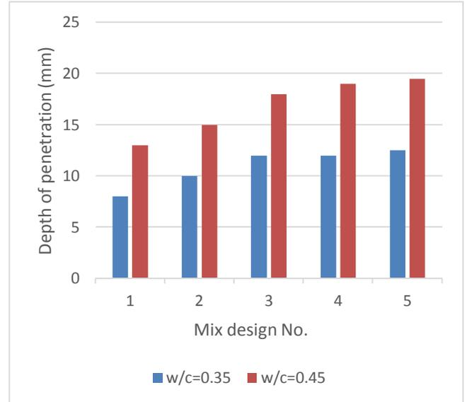
Figure 7. Diagram of variations of water penetration in mix designs vs amount of recycled aggregates
