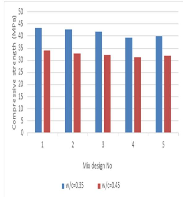
Figure 5. Diagram of compressive strength
