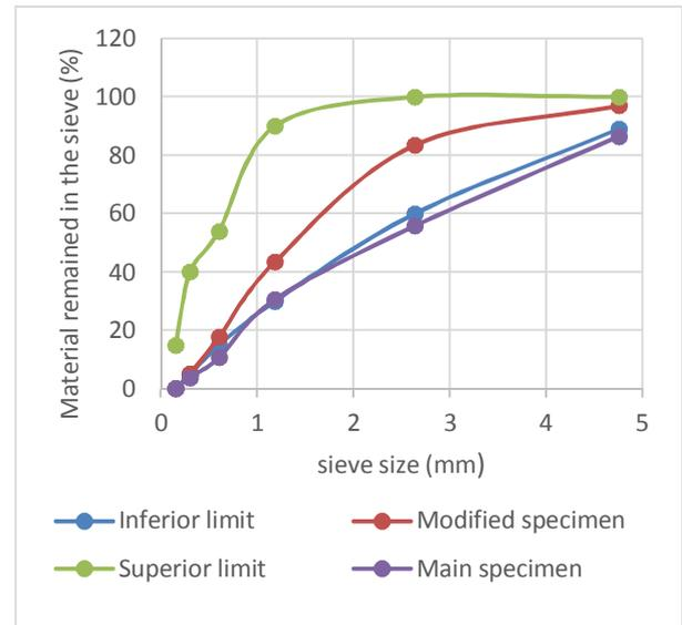
Figure 1. Diagram of sand grading
