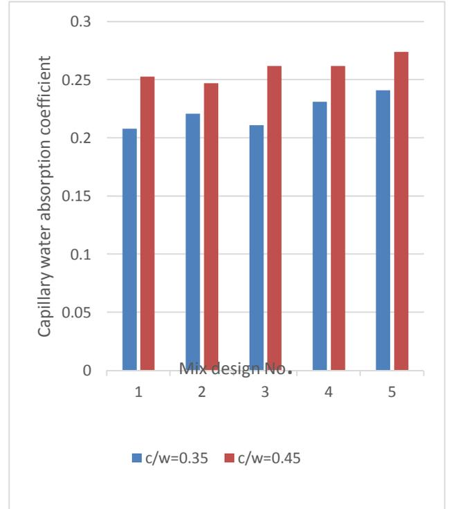
Figure 6. Diagram of variations of capillary water absorption coefficient in mix designs vs increasing the amount of recycled aggregates.
