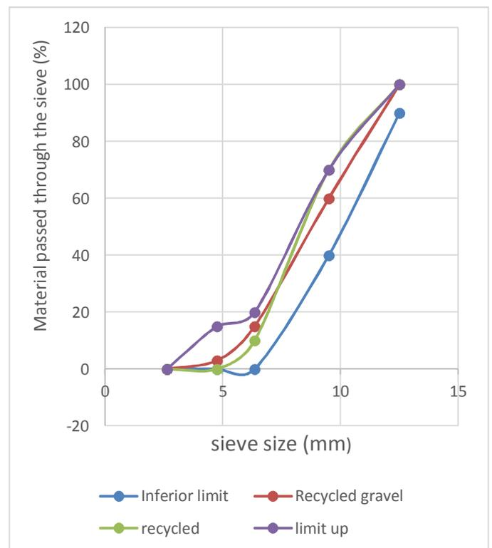
Figure 2. Grading diagram of natural and recycled gravel
