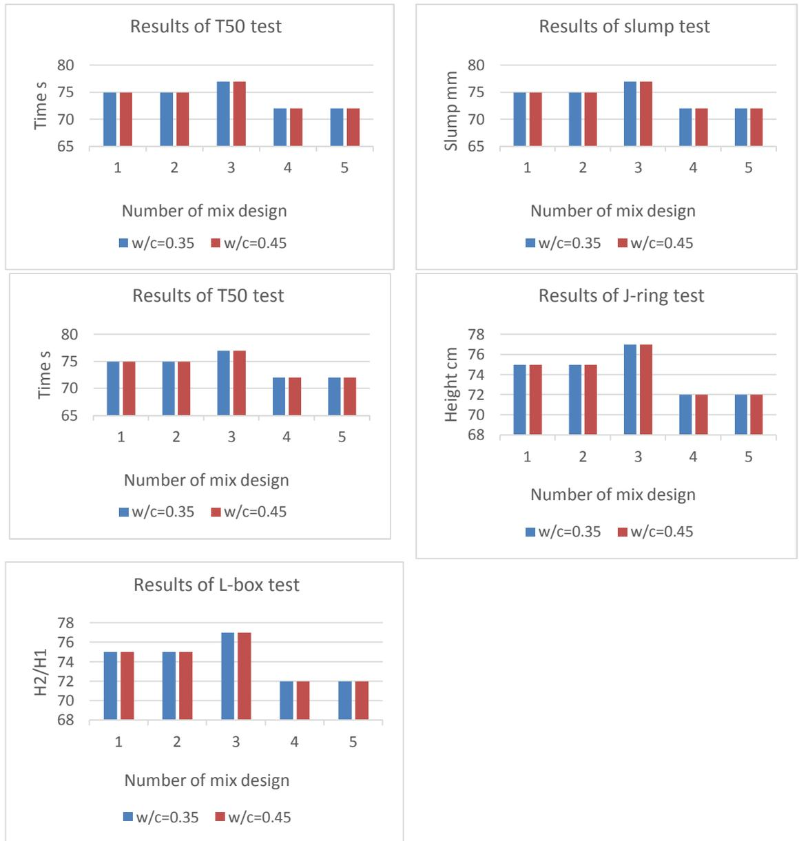
Figure 3. workability tests results on fresh concrete
